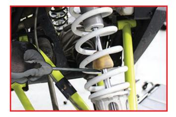
Rotate OEM Preload ring counter clockwise all the way to top of threaded shock body. Use 1/8" punch.
