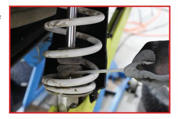
Rotate OEM Preload ring counter clockwise until the OEM spring stack is loose. Use 3/8" punch.
