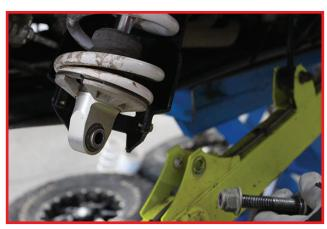
Push up on spring stack to remove OEM lower spring retainer and OEM rock guard.
