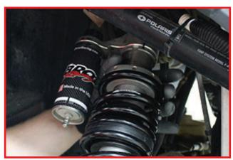
Set compression adjuster knob to mid range. Adjust as needed for driving terrain.
