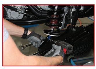
Set "zero Preload" by rotating Preload ring clockwise until spring stack contacts Preload ring.
