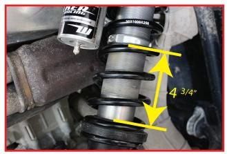
Set compression adjuster knob to mid range. Adjust as needed for driving terrain.
