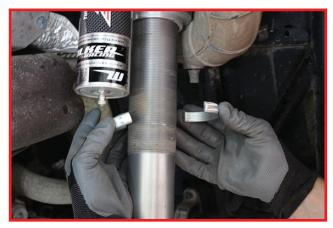
Use 3/32" allen wrench to secure cross over ring to shock body. Do not tighten, you will set final cross over point in final step. \*Make sure cross over ring spins freely to avoid cross threading.
