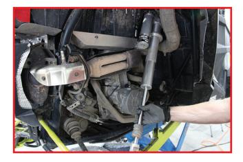
Install new two piece rear billet cross over ring to shock body.
