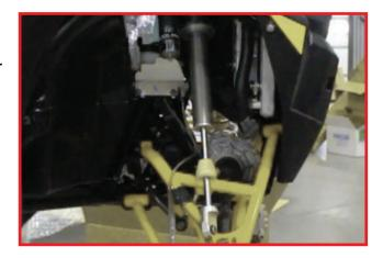
Install new tender spring with progressive or tighter coils towards top. Install new spring divider with long end pointing up.
