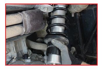
Install new main spring, OEM rock guard and OEM lower spring retainer.
