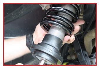
Install new main spring and new lower spring retainer.
