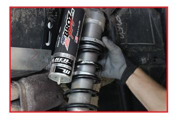
Set cross over ring by measuring 4 3/4" from top of spring divider. Then tighten cross over ring screws.
