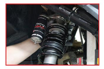
Set "Preload" by rotating Preload ring clockwise an additional 4 full rotations. Use 1/8" punch if difficult to rotate by hand. \*Additional Preload may be needed depending on weight of after-market accessories (bumper, winch, cage, etc).
