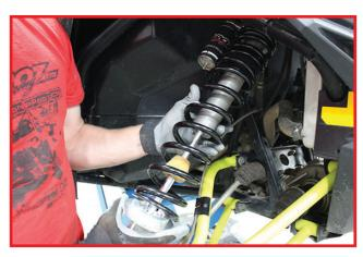
Reconnect shock to a-arm. Torque shock bolt at 42ft-lbs.
