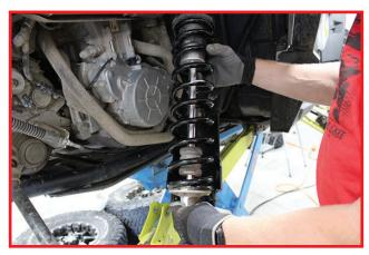
Reconnect shock to trailing arm. Torque shock bolt at 42ft-lbs.
